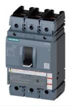
circuit breaker 3VA5 UL frame 250 breaking capacity class H 65kA @ 480 V 3-pole, line protection TM230, FTAM, In=200A overload protection Ir=200A fixed short-circuit protection Ii=5...10 x In UL489 SB (naval), 50 deg. cel. nut keeper kit on both sides
