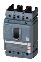
circuit breaker 3VA5 UL frame 250 breaking capacity class H 65kA @ 480V 3-pole, line protection TM230, FTAM, In=200A overload protection Ir=200A fixed short-circuit protection Ii=5...10 x In UL 489 SB (naval), 50° C without connection
