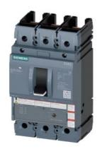
circuit breaker 3VA5 UL frame 250 3-pole, starter protection TM120M, AM, In=200A without overload protection short-circuit protection Ii=3...6 x In without connection
