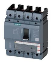
circuit breaker 3VA5 UL frame 250 breaking capacity class C 100kA @ 480V 4-pole, line protection TM230, FTAM, In=175A overload protection Ir=175A fixed short-circuit protection Ii=5...10 x In N conductor unprotected without connection
