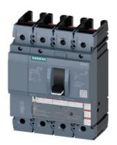
circuit breaker 3VA5 UL frame 250 breaking capacity class C 100kA @ 480V 4-pole, line protection TM240, ATAM, In=150A overload protection Ir=120A...150A short-circuit protection Ii=5...10 x In N conductor protection 100% without connection
