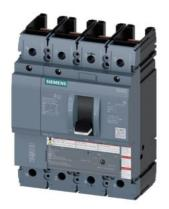
circuit breaker 3VA5 UL frame 250 breaking capacity class C 100kA @ 480V 4-pole, line protection TM210, FTFM, In=150A overload protection Ir=150A fixed short-circuit protection Ii=10 x In N conductor protection 100% without connection
