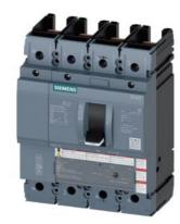
circuit breaker 3VA5 UL frame 250 breaking capacity class C 100kA @ 480V 4-pole, line protection TM230, FTAM, In=150A overload protection Ir=150A fixed short-circuit protection Ii=5...10 x In N conductor protection 100% without connection
