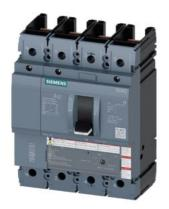
circuit breaker 3VA5 UL frame 250 breaking capacity class C 100kA @ 480V 4-pole, line protection TM240, ATAM, In=150A overload protection Ir=120A...150A short-circuit protection Ii=5...10 x In N conductor unprotected without connection
