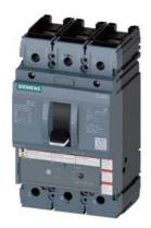
circuit breaker 3VA5 UL frame 250 breaking capacity class C 100kA @ 480 V 3-pole, line protection TM240, ATAM, In=150A overload protection Ir=120A ...150A short-circuit protection li=5...10 x In nut keeper kit on both sides
