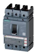
circuit breaker 3VA5 UL frame 250 breaking capacity class C 100kA @ 480V 2-pole, line protection TM210, FTFM, In=150A overload protection Ir=150A fixed short-circuit protection Ii=10 x In without connection
