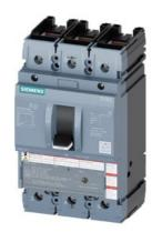
circuit breaker 3VA5 UL frame 250 breaking capacity class C 100kA @ 480 V 3-pole, line protection TM210, FTFM, In=150A overload protection Ir=150A fixed short-circuit protection li=10 x In cable connection on both sides
