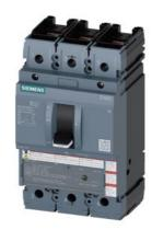
circuit breaker 3VA5 UL frame 250 breaking capacity class C 100kA @ 480 V 3-pole, line protection TM210, FTFM, In=150A overload protection Ir=150A fixed short-circuit protection Ii=10 x In UL489 SB (naval), 50 deg. cel. nut keeper kit on both sides
