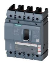
circuit breaker 3VA5 UL frame 250 breaking capacity class C 100kA @ 480V 4-pole, line protection TM230, FTAM, In=150A overload protection Ir=150A fixed short-circuit protection li=5...10 x In N conductor unprotected without connection
