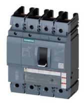
circuit breaker 3VA5 UL frame 250 breaking capacity class H 65kA @ 480V 4-pole, line protection TM240, ATAM, In=150A overload protection Ir=120A...150A short-circuit protection Ii=5...10 x In N conductor unprotected without connection
