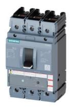
circuit breaker 3VA5 UL frame 250 breaking capacity class H 65kA @ 480 V 3-pole, line protection TM240, ATAM, In=150A overload protection Ir=120A ...150A short-circuit protection li=5...10 x In cable connection on both sides
