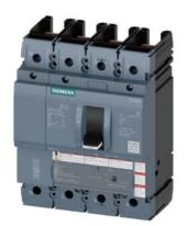
circuit breaker 3VA5 UL frame 250 breaking capacity class H 65kA @ 480V 4-pole, line protection TM210, FTFM, In=150A overload protection Ir=150A fixed short-circuit protection Ii=10 x In N conductor unprotected without connection
