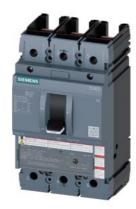
circuit breaker 3VA5 UL frame 250 breaking capacity class H 65kA @ 480V 3-pole, line protection TM210, FTFM, In=150A overload protection Ir=150A fixed short-circuit protection Ii=10 x In UL 489 SB (naval), 50° C without connection
