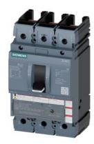
circuit breaker 3VA5 UL frame 250 breaking capacity class H 65kA @ 480V 3-pole, line protection TM230, FTAM, In=150A overload protection Ir=150A fixed short-circuit protection Ii=5...10 x In without connection
