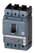
circuit breaker 3VA5 UL frame 250 breaking capacity class M 35kA @ 480 V 3-pole, line protection TM210, FTFM, In=150A overload protection Ir=150A fixed short-circuit protection Ii=10 x In nut keeper kit on both sides
