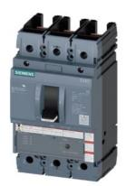
circuit breaker 3VA5 UL frame 250 3-pole, starter protection TM120M, AM, In=150A without overload protection short-circuit protection Ii=3...6 x In without connection
