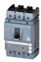
circuit breaker 3VA5 UL frame 250 3-pole, starter protection TM120M, AM, In=150A without overload protection short-circuit protection li=6...12 x In cable connection on both sides
