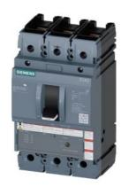
circuit breaker 3VA5 UL frame 250 3-pole, starter protection TM120M, AM, In=150A without overload protection short-circuit protection Ii=6...12 x In nut keeper kit on both sides
