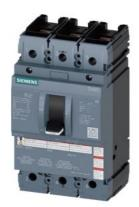
molded case switch 3VA5 UL frame 250 max. sh-circ breaking capacity 65kA @ 480 V 3-pole, line protection MCS110, In=150A without overload protection self-protection li=16 x In nut keeper kit on both sides
