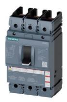
molded case switch 3VA5 UL frame 250 max. sh-circ breaking capacity 65kA @ 480V 3-pole, line protection MCS110, In=150A without overload protection self-protection li=16 x In without connection
