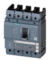
circuit breaker 3VA5 UL frame 250 breaking capacity class C 100kA @ 480V 4-pole, line protection TM240, ATAM, In=125A overload protection Ir=100A...125A short-circuit protection Ii=5...10 x In N conductor protection 100% without connection
