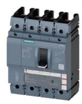
circuit breaker 3VA5 UL frame 250 breaking capacity class C 100kA @ 480V 4-pole, line protection TM230, FTAM, In=125A overload protection Ir=125A fixed short-circuit protection li=5...10 x In N conductor unprotected without connection
