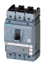
circuit breaker 3VA5 UL frame 250 breaking capacity class C 100kA @ 480 V 3-pole, line protection TM230, FTAM, In=125A overload protection Ir=125A fixed short-circuit protection li=5...10 x In cable connection on both sides
