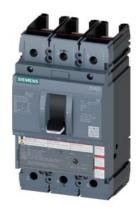
circuit breaker 3VA5 UL frame 250 breaking capacity class H 65kA @ 480V 3-pole, line protection TM210, FTFM, In=125A overload protection Ir=125A fixed short-circuit protection Ii=10 x In without connection
