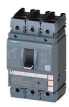
circuit breaker 3VA5 UL frame 250 breaking capacity class H 65kA @ 480 V 3-pole, line protection TM230, FTAM, In=125A overload protection Ir=125A fixed short-circuit protection Ii=5...10 x In nut keeper kit on both sides
