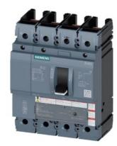
circuit breaker 3VA5 UL frame 250 breaking capacity class M 35kA @ 480 V 4pole, line protection TM240, ATAM, In=125A overload protection Ir=100A...125A short-circuit protection Ii=5...10 x In N conductor protection 100% without connection
