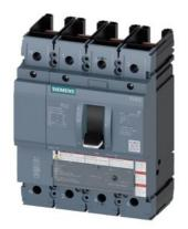
circuit breaker 3VA5 UL frame 250 breaking capacity class M 35kA @ 480 V 4-pole, line protection TM230, FTAM, In=125A overload protection Ir=125A fixed short-circuit protection Ii=5...10 x In N conductor unprotected without connection
