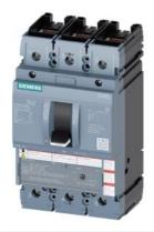
circuit breaker 3VA5 UL frame 250 breaking capacity class C 100kA @ 480 V 3-pole, line protection TM230, FTAM, In=110A overload protection Ir=110A fixed short-circuit protection Ii=5...10 x In cable connection on both sides
