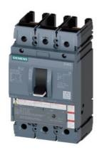
circuit breaker 3VA5 UL frame 250 breaking capacity class C 100kA @ 480V 2-pole, line protection TM230, FTAM, In=100A overload protection Ir=100A fixed short-circuit protection Ii=5...10 x In without connection
