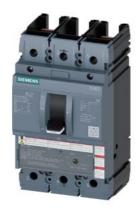
circuit breaker 3VA5 UL frame 250 breaking capacity class H 65kA @ 480V 2-pole, line protection TM210, FTFM, In=100A overload protection Ir=100A fixed short-circuit protection Ii=10 x In without connection
