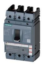
circuit breaker 3VA5 UL frame 250 breaking capacity class H 65kA @ 480V 2-pole, line protection TM230, FTAM, In=100A overload protection Ir=100A fixed short-circuit protection Ii=5...10 x In without connection
