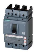
circuit breaker 3VA5 UL frame 250 breaking capacity class M 35kA @ 480 V 3-pole, line protection TM210, FTFM, In=100A overload protection Ir=100A fixed short-circuit protection Ii=10 x In UL 489 SB (naval), 50° C without connection
