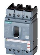
molded case switch 3VA5 UL frame 250 max. sh-circ breaking capacity 100kA @ 480 V 3-pole, line protection MCS110, In=100A without overload protection self-protection li=25 x In cable connection on both sides
