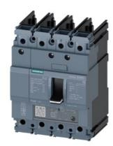
circuit breaker 3VA5 UL frame 125 breaking capacity class S 25kA @ 480V 4-pole, line protection TM240, ATAM, In=15A overload protection Ir=12A...15A short-circuit protection Ii=10...20 x In N conductor unprotected without connection
