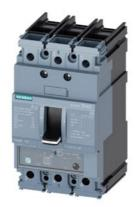
circuit breaker 3VA5 UL frame 125 breaking capacity class S 25kA @ 480 V 3-pole, line protection TM240, ATAM, In=15A overload protection Ir=12A ...15A short-circuit protection Ii=10...20 x In cable connection on both sides
