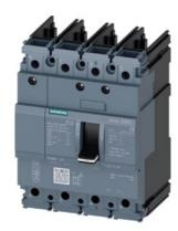
circuit breaker 3VA5 UL frame 125 breaking capacity class S 25kA @ 480V 4-pole, line protection TM210, FTFM, In=15A overload protection Ir=15A fixed short-circuit protection Ii=20 x In N conductor unprotected without connection
