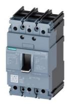
circuit breaker 3VA5 UL frame 125 breaking capacity class S 25kA @ 480 V 3-pole, line protection TM210, FTFM, In=15A overload protection Ir=15A fixed short-circuit protection Ii=20 x In cable connection on both sides
