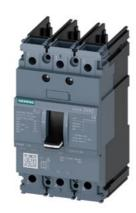
circuit breaker 3VA5 UL frame 125 breaking capacity class S 25kA @ 480V 3-pole, line protection TM210, FTFM, In=15A overload protection Ir=15A fixed short-circuit protection Ii=20 x In without connection
