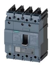
circuit breaker 3VA5 UL frame 125 breaking capacity class S 25kA @ 480V 4-pole, line protection TM230, FTAM, In=15A overload protection Ir=15A fixed short-circuit protection Ii=10...20 x In N conductor unprotected without connection
