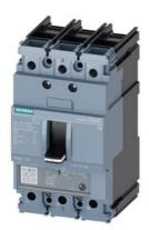
circuit breaker 3VA5 UL frame 125 breaking capacity class S 25kA @ 480 V 3-pole, line protection TM230, FTAM, In=15A overload protection Ir=15A fixed short-circuit protection Ii=10...20 x In UL489 SB (naval), 50 deg. cel. cable connection on both sides
