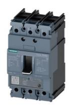
circuit breaker 3VA5 UL frame 125 breaking capacity class S 25kA @ 480 V 3-pole, line protection TM230, FTAM, In=15A overload protection Ir=15A fixed short-circuit protection Ii=10...20 x In nut keeper kit on both sides
