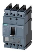
circuit breaker 3VA5 UL frame 125 breaking capacity class S 25KA @ 480 V 3-pole, line protection TM230, FTAM, In=15A overload protection Ir=15A fixed short-circuit protection Il=5...10xIN UL 489 SB (naval),  $50^{\circ}$  cel. without connection
