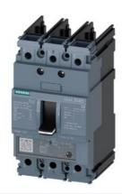
circuit breaker 3VA5 UL frame 125 breaking capacity class S 25KA @ 480 V 3-pole, line protection TM230, FTAM, In=15A overload protection Ir=15A fixed short-circuit protection II=5...10xIN without connection
