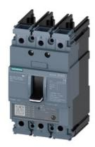
circuit breaker 3VA5 UL frame 125 3-pole, starter protection TM120M, AM, In=15A without overload protection short-circuit protection li=3...7 x In without connection
