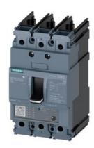
circuit breaker 3VA5 UL frame 125 3-pole, starter protection TM120M, AM, In=10A without overload protection short-circuit protection li=3...7 x In without connection
