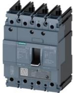
circuit breaker 3VA5 UL frame 125 breaking capacity class H 65kA @ 480V 4-pole, line protection TM230, FTAM, In=90A overload protection Ir=90A fixed short-circuit protection Ii=5...10 x In N conductor protection 100% without connection
